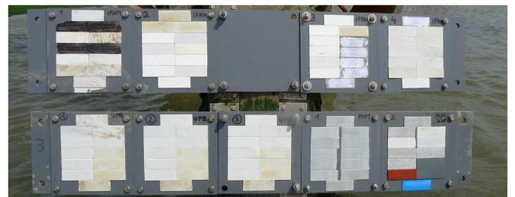
**Fig. 4** Cypris larvae rapid test at the seaside of Norderney with micro slides exposed to field conditions.
